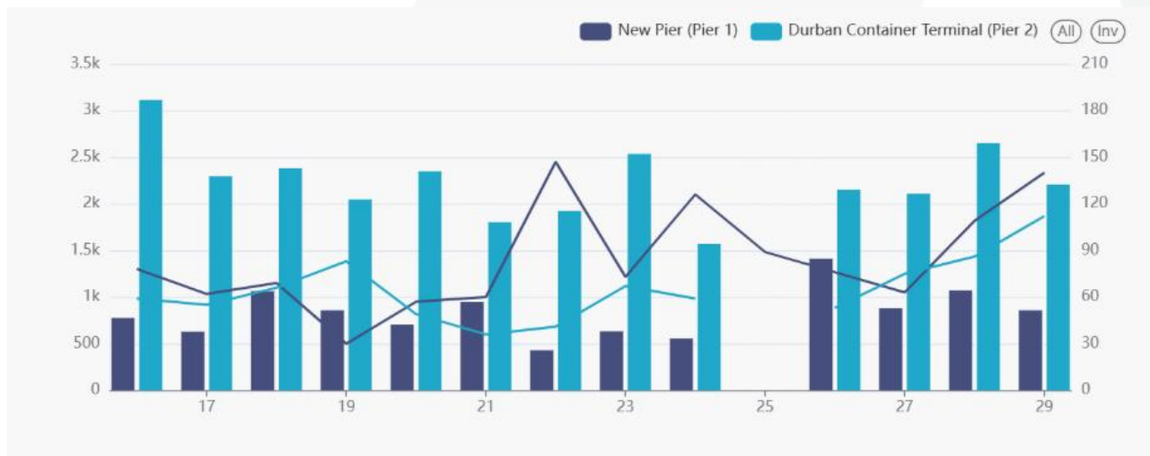
Figure 7 – Gate moves (left axis) and time spent in the terminal (in minutes, right axis)
